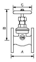
TESTING HYDROSTATIC: BODY: 24 Kg/Cm<sup>2</sup> SEAT : 16 Kg/Cm<sup>2</sup>
