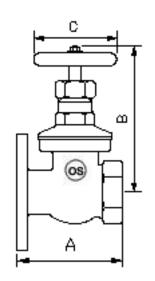
TESTING HYDROSTATIC: BODY: 24 Kg/Cm<sup>2</sup> SEAT : 16 Kg/Cm<sup>2</sup>
